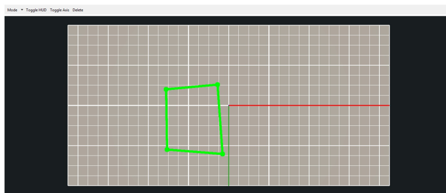
Figure 1.17: A new polygon, colored green because the user has not yet permanently added it to the mesh.
